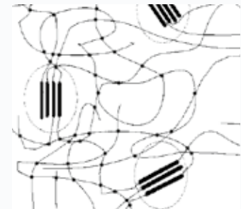
AFTER cross-linking: Schematic representation of chain-forming macromolecules after cross-linking. Three-dimensional cross-linking of polymer chains (heavily impaired freedom of movement).
